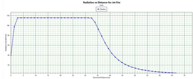
Fig. 6 Jet fire as distance (PHAST 7.11)
